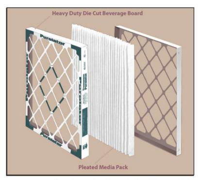
Two mating pieces of die cut beverage board form a double wall frame around all four edges of the filter. Defiant Mark 80-D filters will not rack or warp under normal operating conditions.
